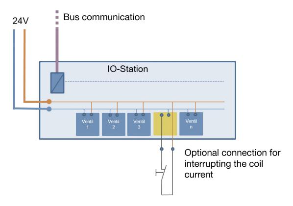
The patented shut-off function is implemented via a second connection via which the power circuit of the solenoid can be interrupted.
