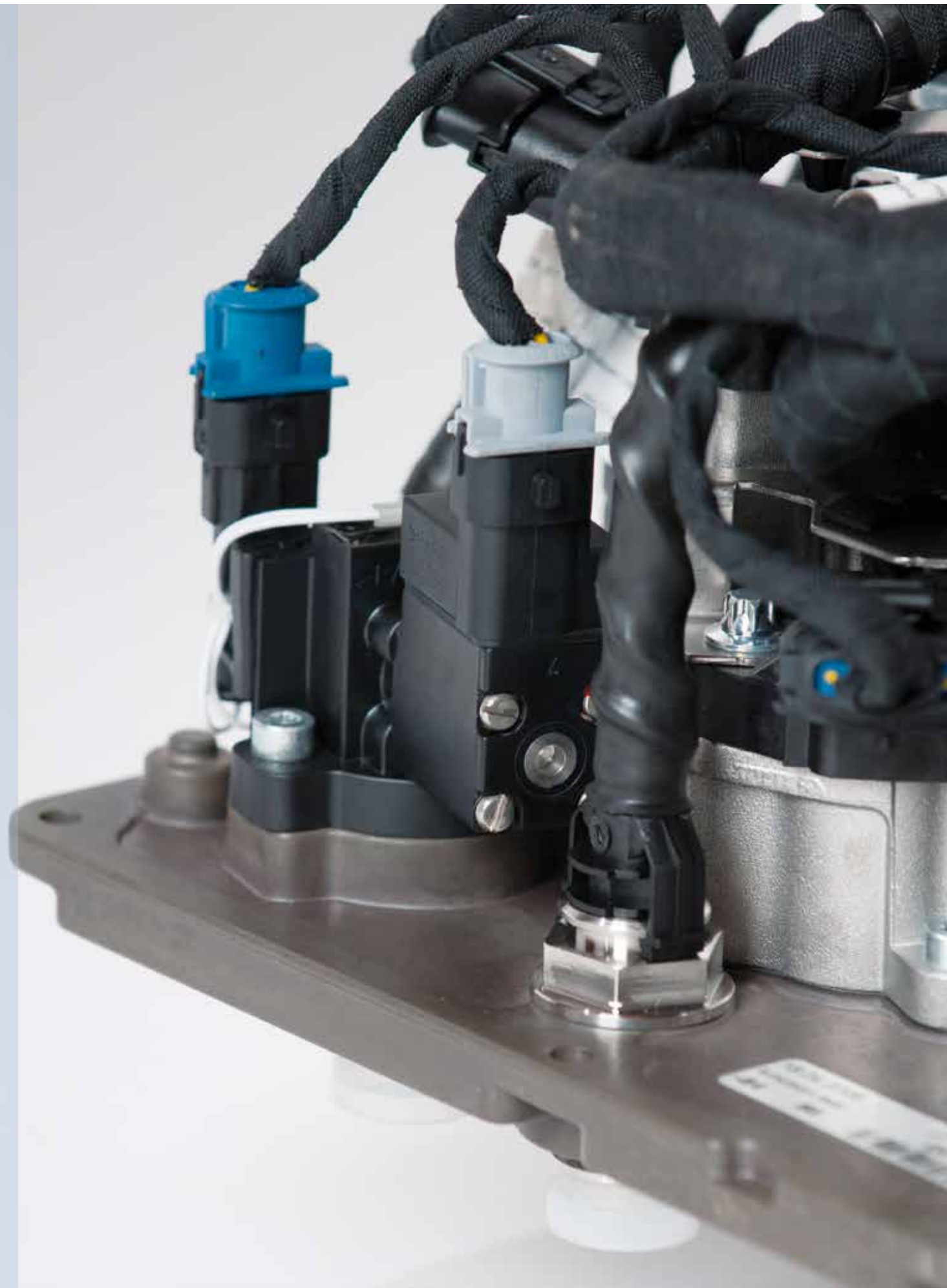
Valve assembly with plastic parts in the SCR aggregate
